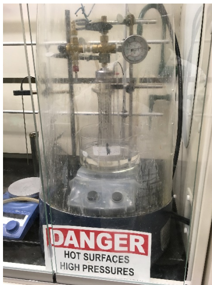
Figure 7. Use a blast shield and post proper signage indicating high pressure!
