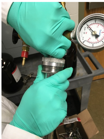
Figure 2. When properly secured, the tube can still rotate around the metal enclosure.
