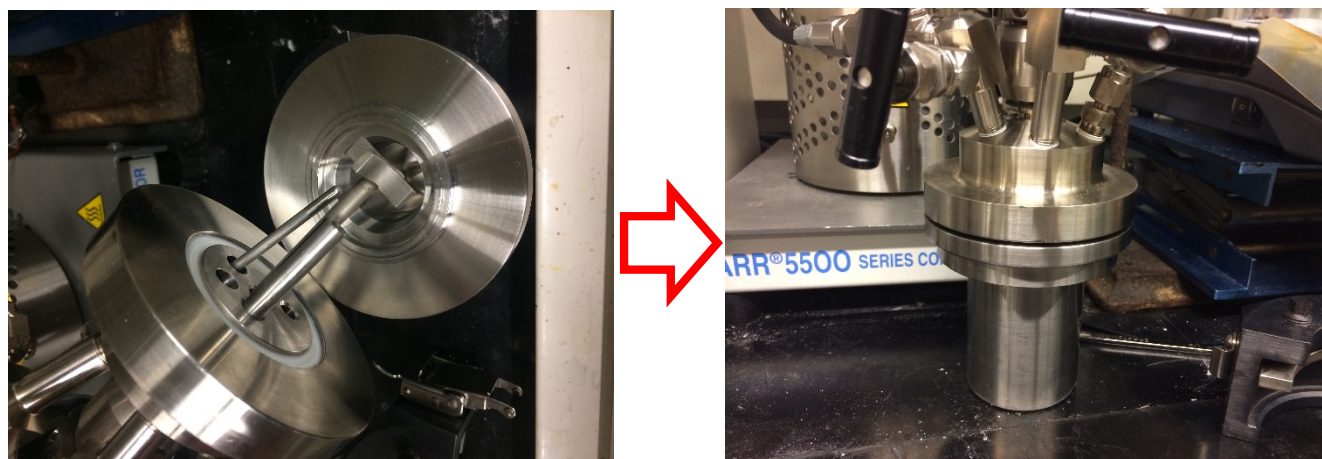
Figure 2. Placing the reactor head on the reactor cylinder.
