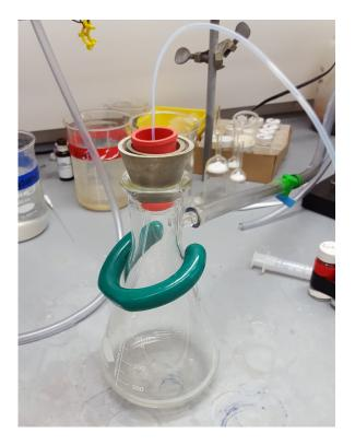
The NMR tube cleaner is assembled by fitting a filter flask with a rubber septum containing a hole for plastic tubing feed-through. After opening the flask to vacuum, the NMR tube is placed over the tubing, resting on top of the septum. The top of the septum is sprayed with acetone, which rinses the NMR tube and drains through the
