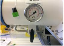
Refill the large antechamber with nitrogen by opening the yellow valve. Note:
