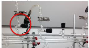
9. Open the crossover valve to pump down the back manifold up to the needle valve on the regulator. Note: If a crossover valve is not available, place a cap on one of the ports of the Schlenk line and open both valves (gas and vacuum) to pump down the back manifold.
