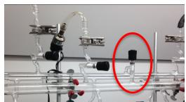
10. Close the crossover valve. Open the cylinder valve and adjust the regulator to ~15-20 psi using the regulator dial. Close the cylinder valve. Open the needle valve to fill the back manifold with CO, then close the needle valve.
