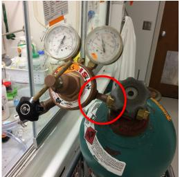
8. Once the regulator connection has been tested for leaks, close the special (usually inert gas) gas inlet valve and ensure the needle valve on the regulator is closed and the gas port leading to the gas manifold is open.
