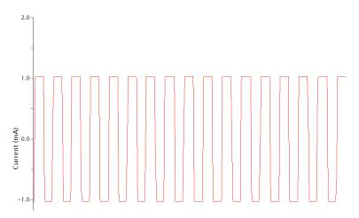
An example of slightly too much iR comp. Note that the current axis is inverted here, but is of similar magnitude to the previous example of a "good" iR comp value
