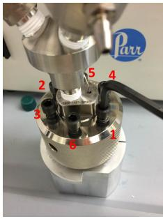
Close the needle valves in the vessel head.
